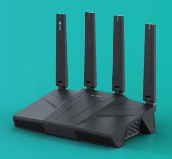
Flint 3e (GL-BE6500) is a high-performance dual-band Wi-Fi 7 router designed to deliver ultra-fast and reliable connectivity for homes, professionals, and small to medium-sized businesses. With combined speeds up to 6500Mbps (688Mbps@2.4GHz + 5764Mbps@5GHz) and Multi-Link Operation (MLO) technology, it ensures seamless cross-band performance and optimized network efficiency.
