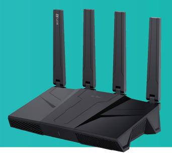
Flint 3 (GL-BE9300) is a tri-band Wi-Fi 7 home router delivering a combined speed of up to 9300 Mbps (688 Mbps @ 2.4GHz, 2882 Mbps @ 5GHz, 5765 Mbps @ 6GHz), featuring MLO technology for seamless multi-band connectivity. Equipped with five 2.5G Ethernet ports, including four supporting 10Gbps aggregation, ensuring ultra-fast wired performance.
