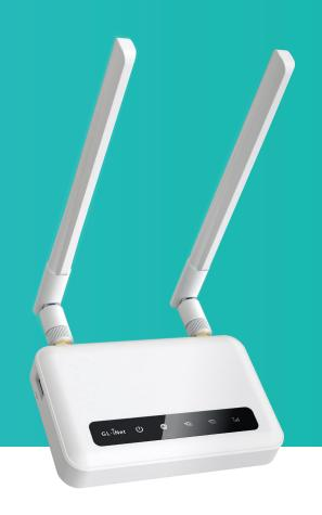
Spitz (GL-X750/GL-X750V2) is a 3G/4G dual-band wireless router, widely used for smart home and IoT areas. Running OpenWRT OS, you can compile your firmware to fit different application scenarios. It has a built-in mini PCIe 3G/4G module to support different operators and can be used all over the world.
