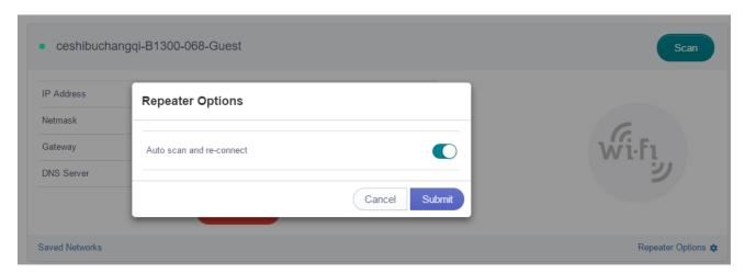
Auto scan and connection: It enables auto switching to available SSID.
