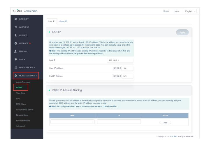
LAN IP: Set router LAN IP address
