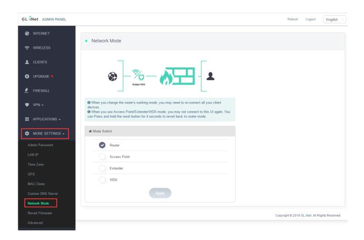
Routing mode: The device connect to upper device by WAN Port, repeater, tethering or modem.
