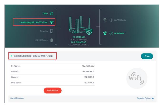
SSID, IP address, subnet mask, gateway, DNS server will be displayed.
