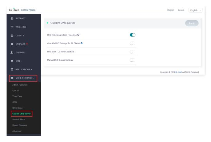
DNS re-binding attack protection: on/off is optional, default on
