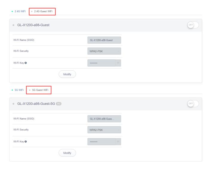
Guest WiFi is turned off in default. Modification of wireless network name, wireless network security, and wireless network password is supportable.
