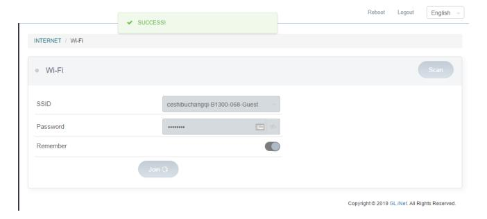
Wait 5s, it will enter into admin panel. Status bar will show the SSID connected, showing as below:
