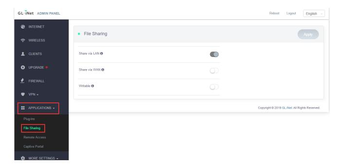
File sharing by LAN: Share to LAN in default, USB flash disk and SD card can be accessed through LAN IP.
