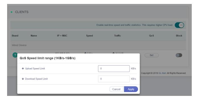
The speed limit value can be checked. Click Reset to cancel speed limit, showing as below:
