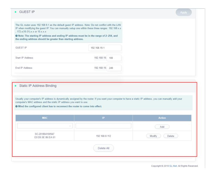
Note: Static binding requires client to retrieve IP.
