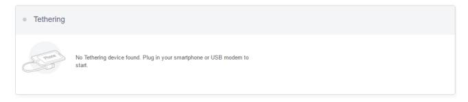
Use original USB cable to connect phone and the device, then turn on USB network sharing of the phone, showing as below:
