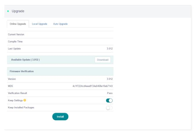
Configuration upgrade is kept in default. Click 'Install' to start updating firmware. Please do not cut off power during the process, otherwise the device is unable to start.
