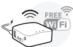
Using **Repeater** means connecting your mini router to another existing wireless network, e.g. when you are using Wi-Fi in hotels or other public locations.
