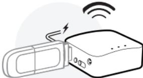
Plug your 3G/4G modem into the USB2.0 port of the router, and it can transfer the 3G/4G signal to Wi-Fi.
