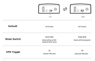
() By default, the switch button has no function. You need to enable above functions manually on the web interface (Available in our firmware v2.26 +).
