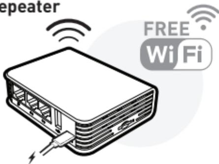
Using **Repeater** means connecting your mini router to another existing wireless network, e.g. when you are using Wi-Fi in hotels or other public locations.
